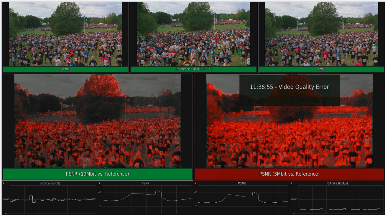
Sample screenshot showing video live quality measurement (LiveQM) with R&S®PRISMON (© video image content: Sveriges Television AB)
