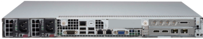
RD9000 rear panel – HDMI &amp; 12G SDI output
